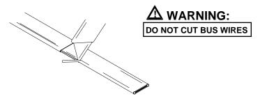
Shave the core material from the outside of each bus wire.
