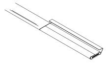
**3** Remove the jacket from the heater cable.
