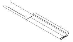
**3** Remove the jacket from the heater cable.
