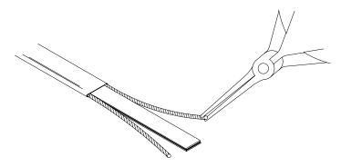
**5** Starting at the end, pull each bus wire away from the core material.
