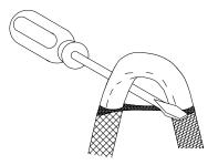
**3** While bending the heater cable, work it through the braid opening.
