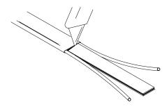
**6** Remove exposed core material.
