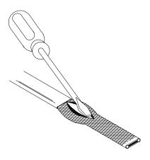
**6** At the bulge, separate the braid to make an opening.
