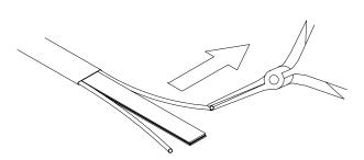
**5** Starting at the end, in the same plane as the cable, pull each bus wire away from the core material.
