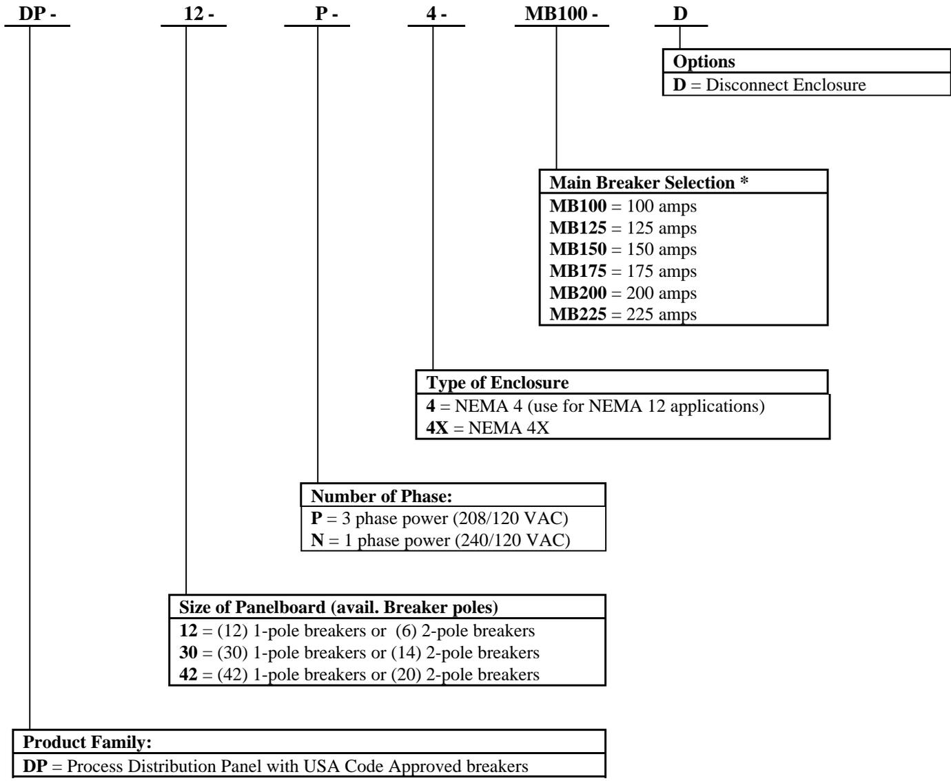
\*Note: Standard 12-Pole option is limited to 100A maximum main breaker sizing.
