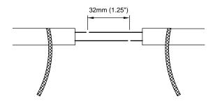
• Position both heater cables with the ground braid on the same side. Remove 32mm (1.25") of bus wire from each heater cable to offset for insulated splice connectors.
