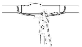
If necessary, cut excess length from braid straps. Crimp the braid straps together into an uninsulated splice connector.
