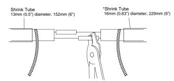
Slide one 18mm (0.7") diameter, 152mm (6") length shrink tube over one of the heater cables. Crimp an insulated splice connector to each bus wire connecting the two heater cables together.
