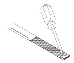
Using an awl or other sharp pointed device, unravel the braid from the cable. Even though most of the outer jacket will be removed in a subsuquent operation, do not puncture it with the awl.
