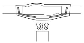
Center the 28mm (1.1") diameter, 229mm (9") length shrink tube over the splice and braid connection. Shrink with heat gun until completely shrunk. A uniform bead of glue should appear around the ends of the shrink tube.
