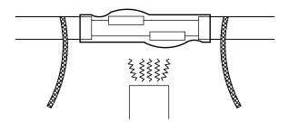
Center the 18mm (0.7") diameter, 152mm (6") length shrink tube over the connectors leaving the braid straps exposed. Shrink with heat gun until completely shrunk. A uniform bead of glue should appear around the ends of the shrink tube.
