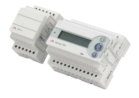
The devireg<sup>™</sup> 850 is the most optimal solution for keeping an area free of ice and snow. devireg<sup>™</sup> 850 acts on information received from the sensor(s) which register both temperature and moisture. devireg<sup>™</sup> 850 calculates the information and secures that the heat only will be turned on when the right combination of low temperature and a certain level of moisture are detected. This gives an energy saving system and reduces running costs.
