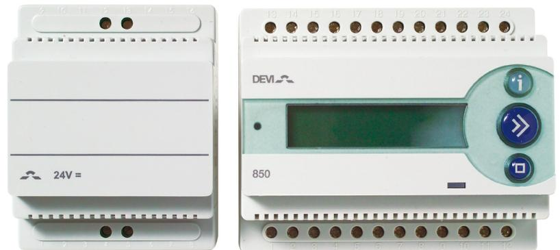
The Devireg™ 850 is the most optimal solution for keeping an area free of ice and snow. Devireg™ 850 acts on information received from the sensor(s) which register both temperature and moisture. Devireg™ 850 calculates the information and secures that the heat only will be turned on when the right combination of low temperature and a certain level of moisture are detected. This gives an energy saving system and reduces running costs.
